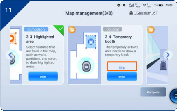
Click "Skip" in the [Temporary Booth] card to suspend the temporary booth function.
