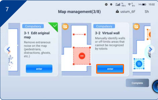
Click "Enter" in the [Virtual Wall] card to add virtual walls to all locations on the map where virtual walls need to be drawn. Please refer to: How to use virtual wall editing.
