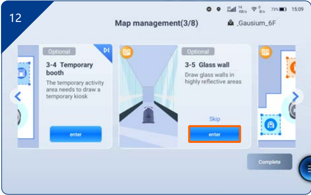
When there are glass walls or other highly reflective walls on site, click "Enter" in the [Glass Wall] card to draw a glass wall at the location of the wall. Please refer to: How to use glass walls . When the target wall does not exist on site, click "Skip".
