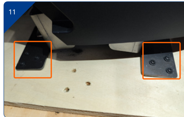
Remove the limiting sheet metal parts that secure the left and right wheel hub motors. There are 6 screws on the left and right wheels.
