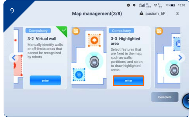
Click "Enter" in the [Highlight Area] card to add highlight areas to all locations on the map where highlight areas need to be drawn. Please refer to: How to use highlight areas.
