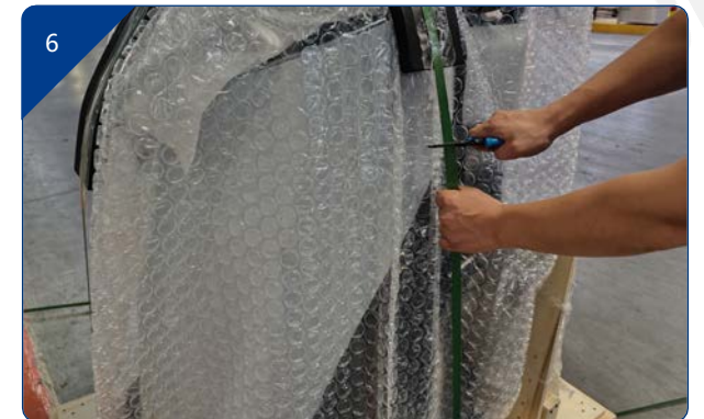
6 Cut off the ties holding the machine in place.
