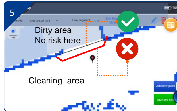
In order to ensure the edge effect of the clean area, when drawing a line segment virtual wall, if there is no risk of falling or scratching, it must be drawn along the outer edge of the clean area as much as possible. If there is a risk, safety first.
